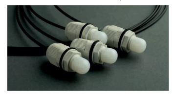
Sensors are characterised by a suitable light absorption coefficient. The sensitivity of the light detection path is set individually depending on the length of the sensors and the conditions in the object. The sensitivity must be selected so that the system does not react to sunlight or headlights used by the operator. The standard lengths of light guides with sensors are 3, 5 and 15 metres respectively.
